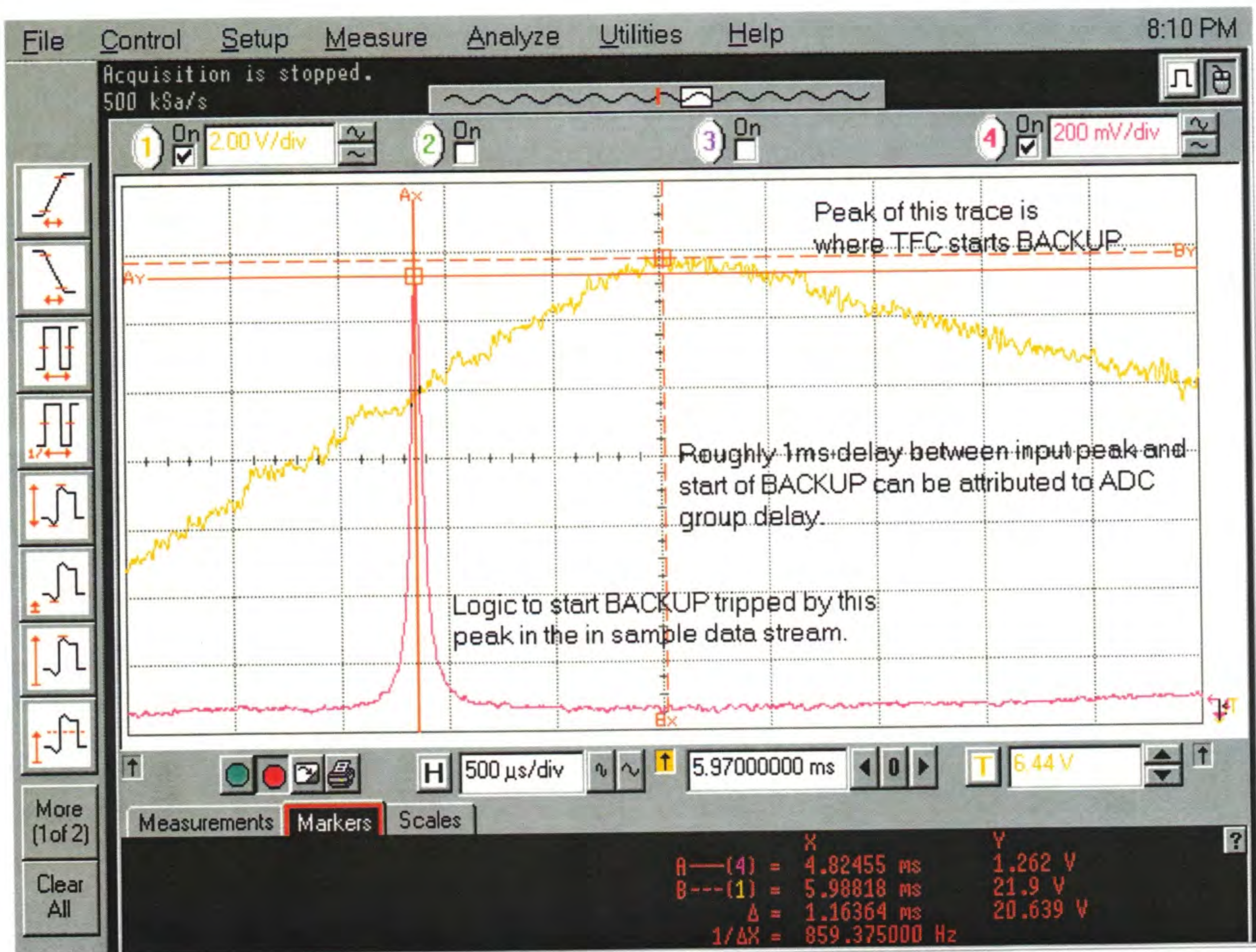
Figure 8: ADC group delay impact on open-loop performance.
